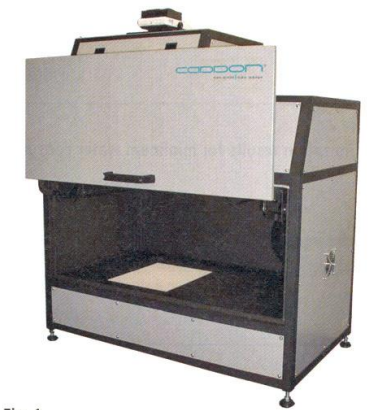
Fig. 1 The measuring system can:scan renders colortrue digital patterns of structured textiles
